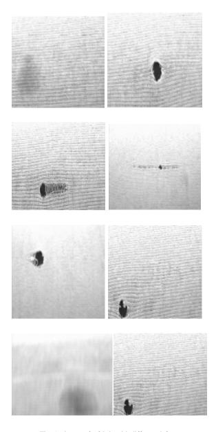
Fig: An image of a fabric with different defects
